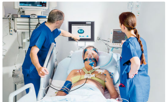
Real-time EIT monitoring during mechanical ventilation with an easy-to-use sensor belt (picture source: swisstom.ch)
